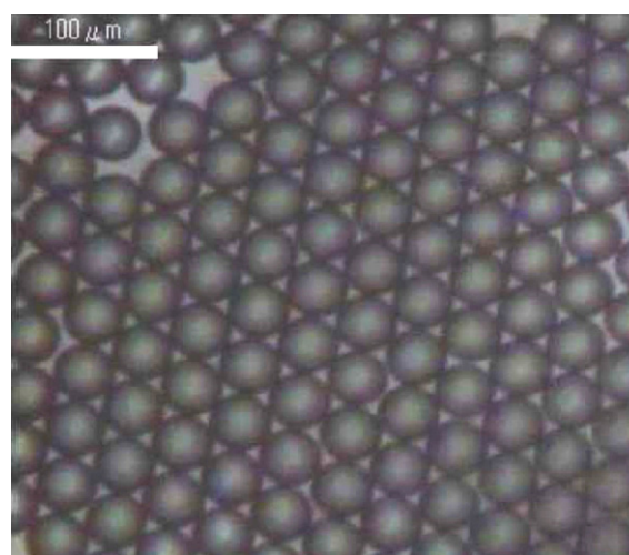
Fig. 1. Protein-stabilized monodisperse emulsion fabricated using the straight-through micro-channel emulsification technique. Reproduced from [13 * ], with permission.
