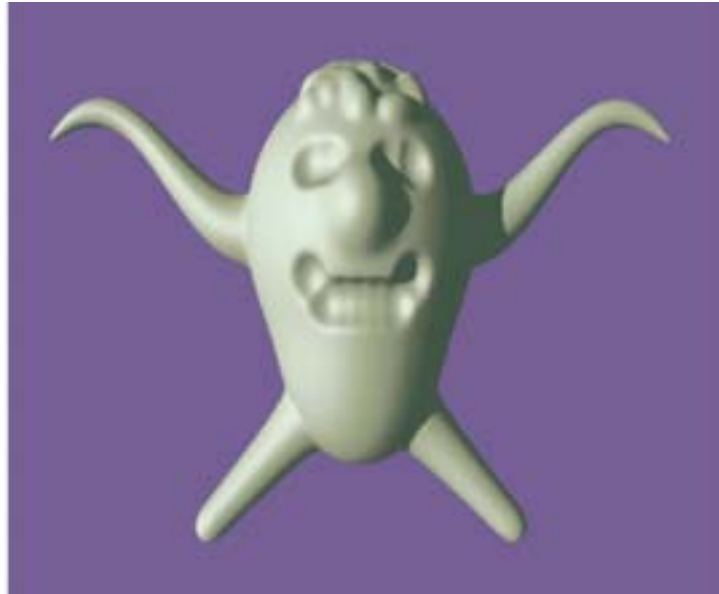
Figure 5.20: Example of the deformation using space mapping. Eyes, nose, mouth, bumps and bottom horns result from point to point based deformations, and top horns are obtained as sets of deformations along a sampled curve.
