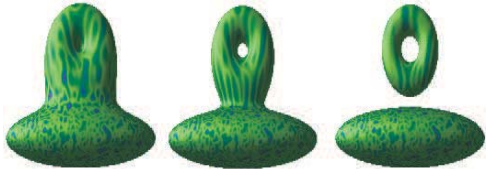
Figure 5.15: Changing the area of influence and \vartheta . The Z function is defined as a FRep tree composed of an intersection of a block and a torus. The parameter varies in a similar way as in eq. 5.14.
