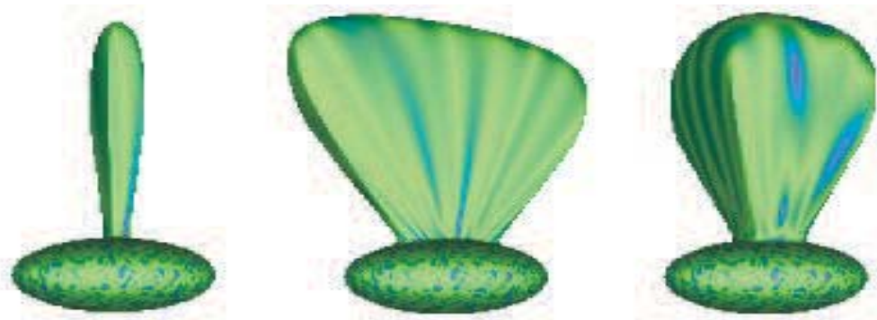
Figure 5.16: Changing the area of influence. The Z function is defined as a FRep tree composed of a tapering operation and a block primitive. From left to right, the first figure shows the initial deformation, then a tapering operation along one axis, and then along two axes.
