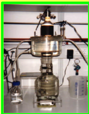
Fig. 1. Benthic Gradient Chamber device (Pringault et al., 1996, FEMS Microbiol. Ecol. 20:237-250).
