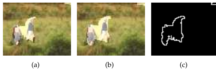
Figure 3.23: Example of an inaccurate segmented object of the sequence “Hiragasy”: (a) The inaccurate segmented object, (b) the object with a dilated mask (1 pixel), (c) the object corona (1 pixel width).
