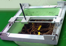
Figure 2: Device to measure x, y, z coordinates of root segments.
