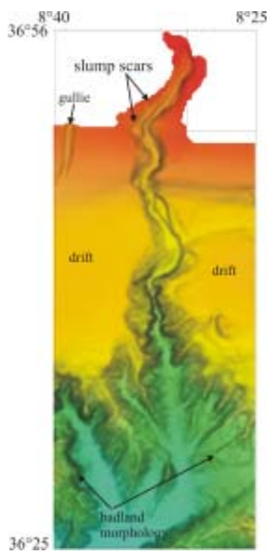
Figure 12. Bathymetric map of the Portimao Canyon and neighbouring valleys. Note the typical badland morphology of the sidewalls suggesting intense gravitational erosion. See Fig. 4 for location.
