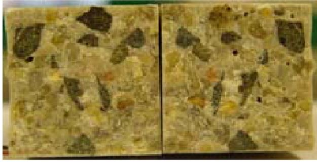
Figure 4.18. Surfaces de rupture flexion 4 points. Éprouvette Car8.
