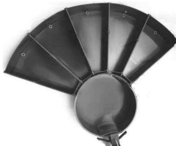
Fig. 1. The five-arm maze. Photograph of the five-arm maze in the configuration used for testing spatial working memory in mice (see Durkin et al., 2000b for details).
