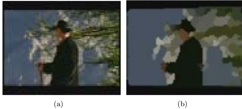
Figure 3.13: in a) a DC frame and in b) the spatial segmentation obtained. Each region has been represented with its average color.
