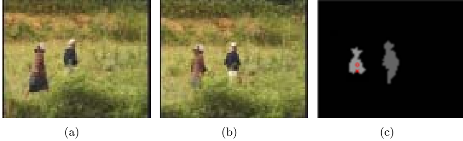
Figure 4.9: Example of wrong object center of mass caused by a partial object detection.
