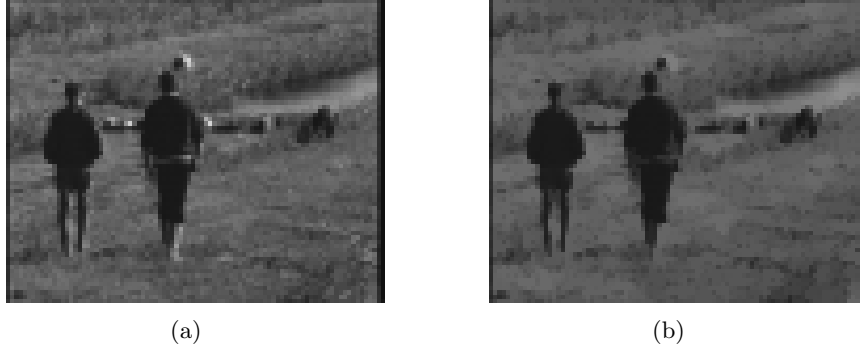
Figure 3.11: a) Y component of a DC image; b) the same DC image after the application of the opening filter.
