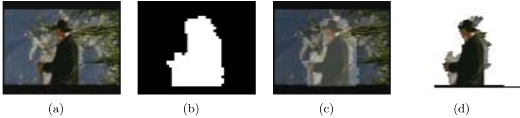
Figure 3.14: a) the original DC image; b) the extracted motion mask; c) merging of the two results and d) the foreground object obtained with this method.
