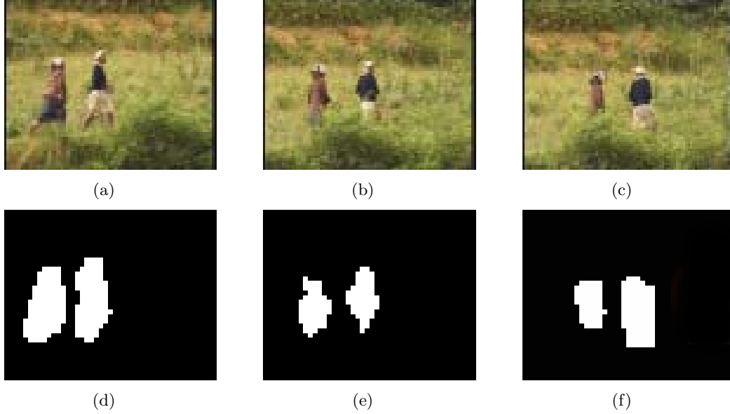
Figure 3.10: On the first row a sequence of I frames and on the second row the extracted object masks.
