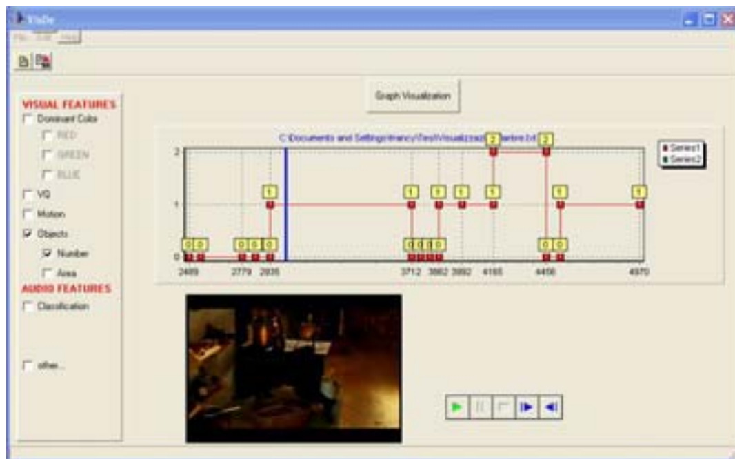
Figure 5.3: An error on the object extraction method occurred: in the graph, where the results of the extraction method are represented, it is possible to see that the extraction method has found an object; this is not true as it appears in the corresponding frame of the video sequence.
