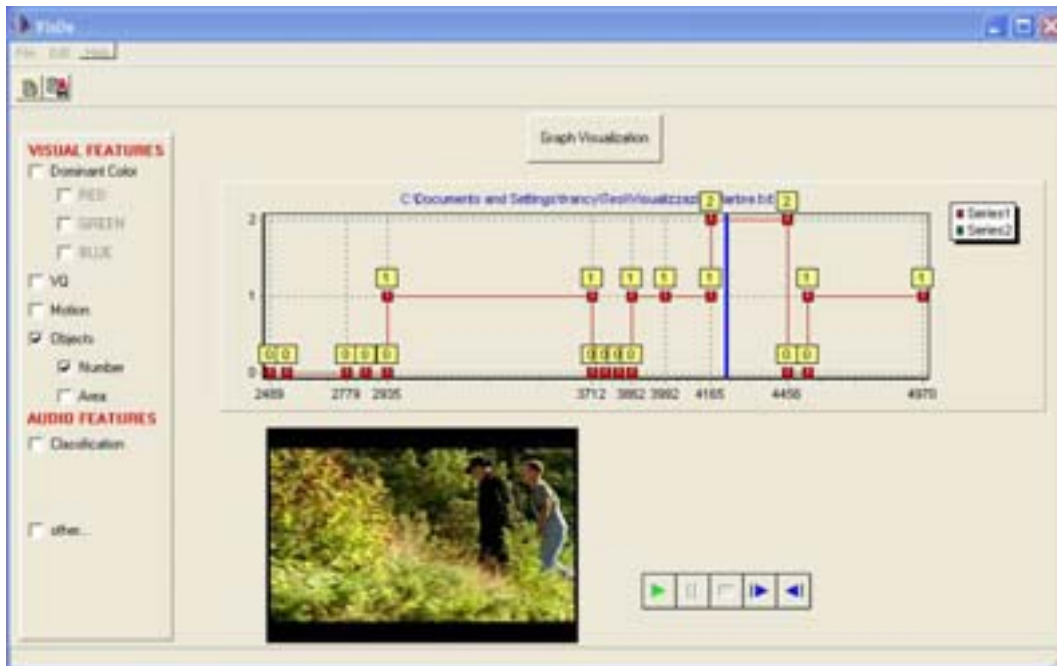
Figure 5.4: The graph shows that our detection algorithm has found two objects in the video sequence. The result is correct in fact in the video sequence we can see two men walking.
