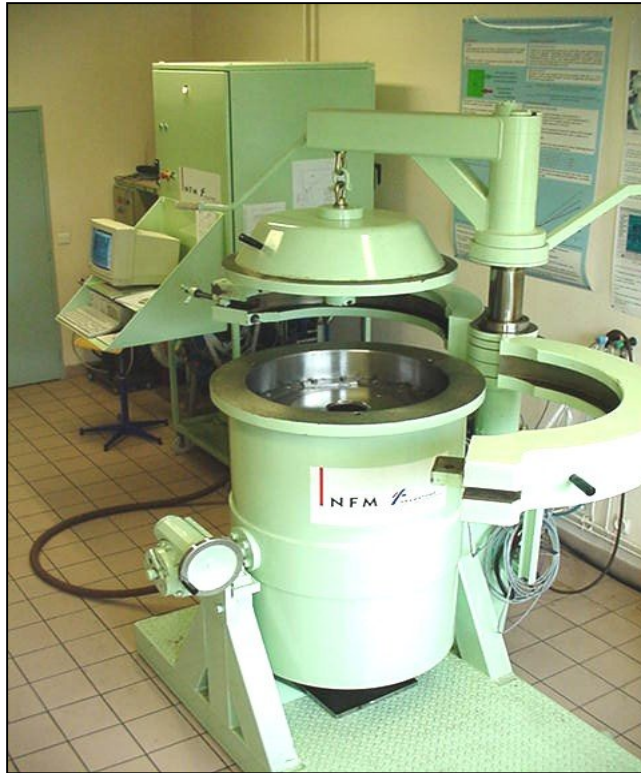
Fig. 12: Apparatus for producing isostatic pressure through direct compression developed at the M.H.P.
