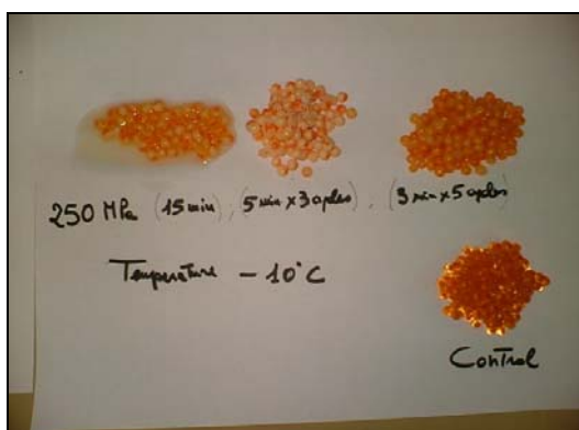
Fig.22 Trout caviar after 250 MPa at -10°C.
