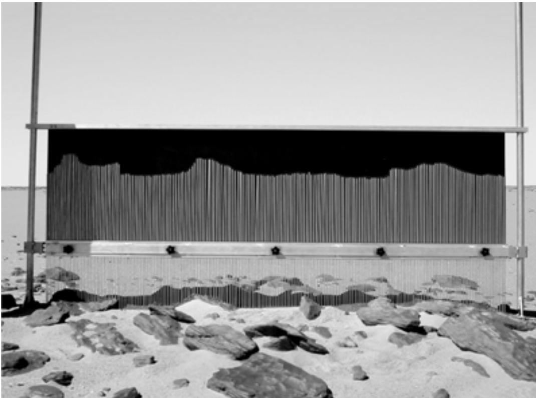
**Figure 3.8 : Sandstone outcrops of the Gifl Kebir formation corresponding to site #3 (top, facing to North, scale given by the foreground tire track) with corresponding surface roughness measurement (bottom, the template is 2 meters long).**
