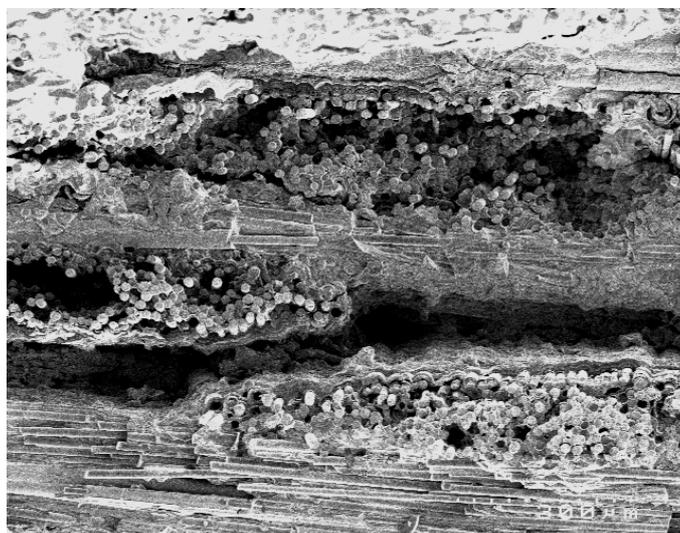
Figure 6 : SEM representative fracture surface of a non-brittle rupture on the C410 specimen exposed for 611 hours at 600°C and 1 MPa in an Air/Steam (80/20) gas mixture.
