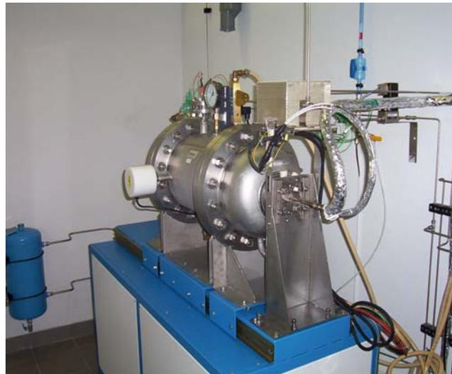
Figure 1b. Picture of the high temperature - high pressure corrosion test equipment
