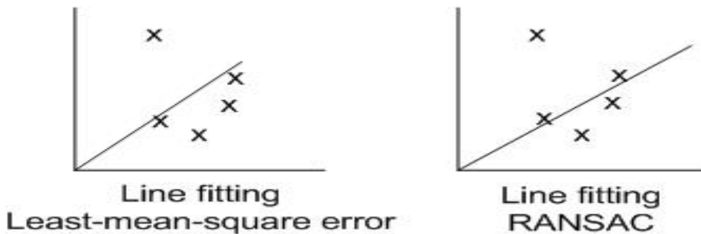
Figure 21. Line fitting methods for camera motion analysis.
