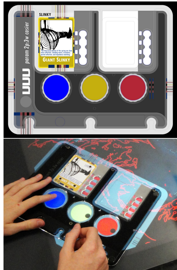
Figure 2. Views of new param casier. This casier currently operates on Microsoft Surface, Apple iPad, and Wacom Bamboo Fun (multitouch+pen), and likely is compatible with numerous other platforms. a) View from design software. A graphical “halo” is visible surrounding all detected tangibles, with cartouche and casier colorbars graphically “extruded” as an indication the correct artifact is detected. b) View as placed upon Microsoft Surface. Three rotary “slotted widgets” are present. In Figure 1c, these are pictured with Surface-tagged wheels inserted. Here, they are pictured with touch interaction bounded by the passive haptic constraints. Two cartouche pads are present, each with four adjoining button/slider slotted widgets. The left pad is occupied by a cartouche. All interactors are placed so as to allow functionality on the sensing surfaces of both the iPad and Bamboo. RFID sensing by supporting electronics is being realized from underneath the Bamboo, and alongside the iPad. The three holes at the bottom of the casier facilitate storage within a traditional three-ring binder.
