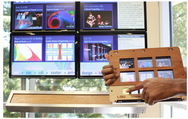
Figure 8. iPad-backed casier in use with a tiled display: Six upper casier regions (illuminated and sensed by the integrated iPad tablet) are used to select presentation options upon the tiled display. A line of six lower casier regions allows selection of which screen is displayed (paralleling content on the tiled display’s lower border). The tile display includes an integrated G8a-format (4.3”×33”) casier, upon which cartouches expressing alternate screen content and behaviors can be placed.
