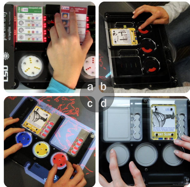
Figure 1. Casier operating across different platforms: (a) standalone tray from [20]; (b,c,d) casier on Apple iPad, Microsoft Surface, Wacom Bamboo Fun – systems marked by diverse sensing, display, and cost. This is prospectively compatible with many other interactive systems.
