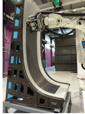
Fig. 18: Robot and landing gear door mold.
