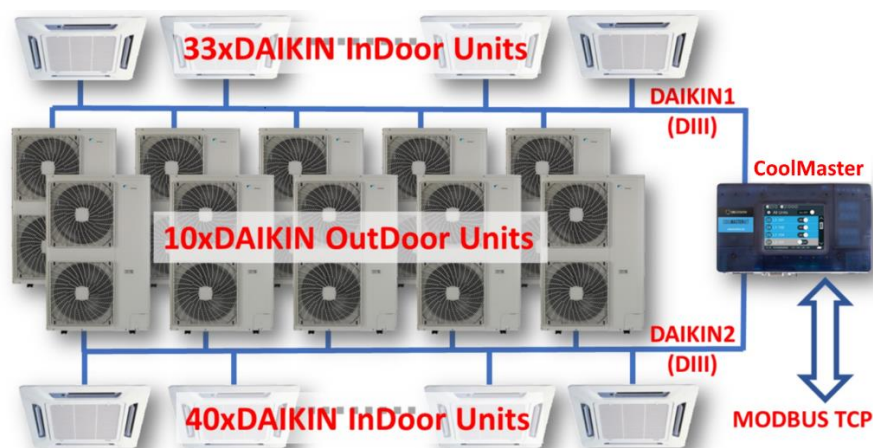
Figure 4. External and internal units of the ESTIA2 HVAC system.
