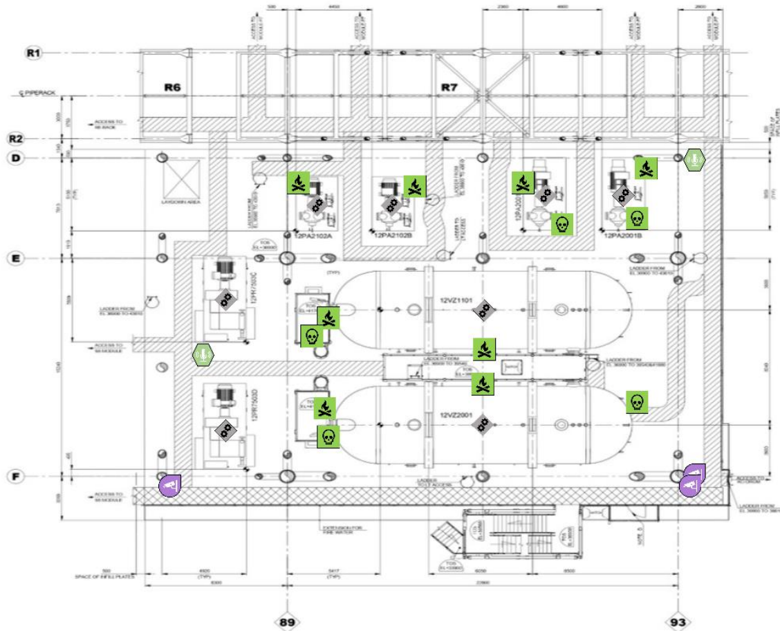
Figure 6 - View of the process deck of the section containing the high-pressure separator and safety equipment selected as the use case
