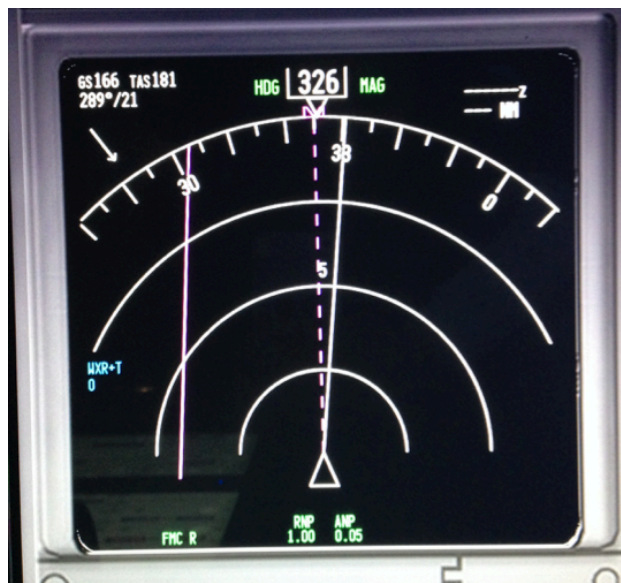
Figure 2. Classical commercial aircraft's navigation display. The left vertical line is the initial trajectory. The right one is the offset. The pilot estimates the distance between these two lines, here about 3 NM.
