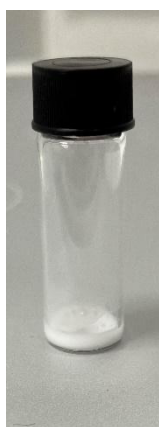
Figure S7. Picture of ELP-g-Bu emulsion with a volume of 100 \mu\text{L} prepared in a glass vial of 4 mL.
